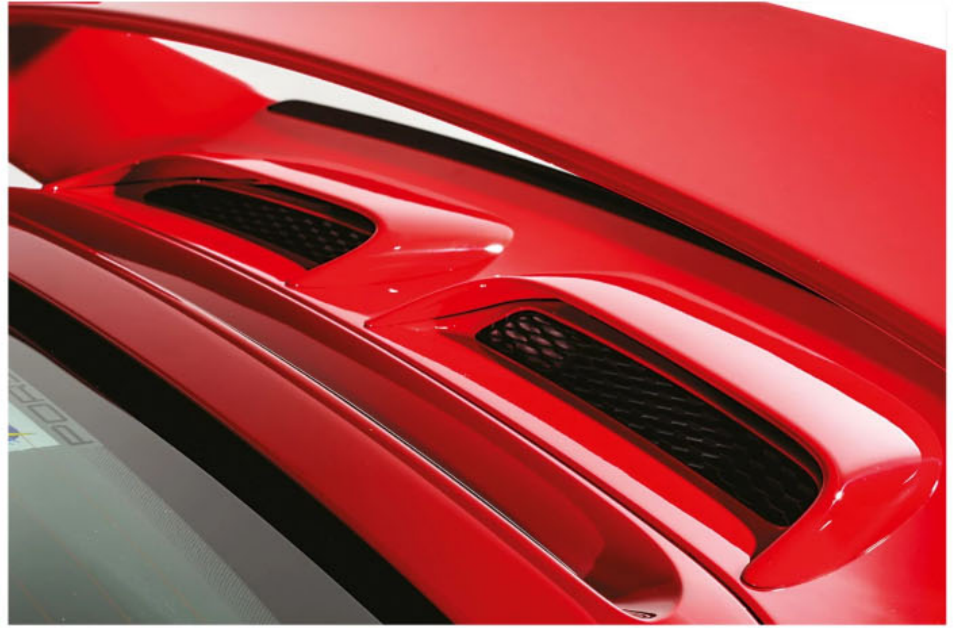
A variety of gills in the rear of the GT3 helped dissipate heat from the high-revving, dry-sump Mezger engine
